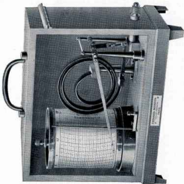
FIG. 12.—Spiral and helical Bourdon tubes. (a) Spiral Bourdon tube; (b) Helical Bourdon tube.
