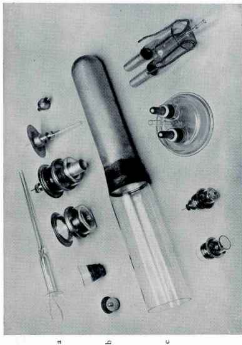
Fig. 38—Some typical copper-to-glass seals, showing (a) "pinch type, utilizing copper-clad wire, as used in filament lamps; (b)–(f) Housekeeper "thin-edge" types, as used in (b) transmitting valve, showing component parts (c) transmitting valve anode, (d) detector valve showing anode and grid discs (e) 5 kW bi-post studio lamp, (f) 5 kW lighthouse lamp.
